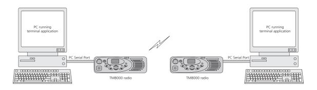
When in Command mode, commands and response messages are passed between the PC and the TM8100 using the CCDI protocol. The Command mode baud rate is selectable using the TM8000 Programming Application to either 1200, 2400, 4800, 9600, 14400 or 19200 baud.
